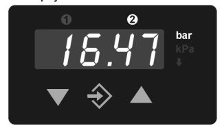
The 3½ digit LED display normally indicates the current pressure. The back-lighted symbols to the right of the digital display indicate the chosen measuring unit. (Note: the units shown in the illustrations of this document can differ from those of the actual instrument). The two LEDs • above the digital display respectively indicate the status of the two limit relays / solid state switches (LED on = relay contacts closed / solid-state switch on).
