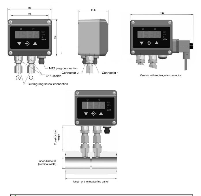
A The dimensions of the measuring panel, in particular the construction height and overall length, are stated in the data information sheet and are recalculated for every application.
