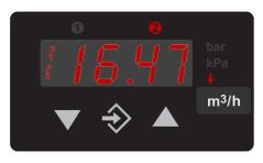
The 3½ digit LED display shows the current flow in normal mode. The unit selected according to the order code is shown on the right of the display. Above the display, two LEDs **0 2** symbolise the status of the switch outputs.
