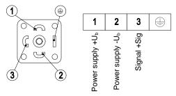
No switch outputs are possible in models with rectangular connectors.
