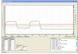
With NS01 Software for Parametrising the level measurement limit switch can be adapted easily and steadily for use with nearly all appropriate media.
