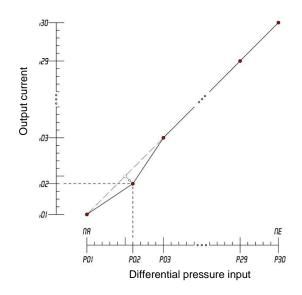
The table comprises 3...30 value pairs. For devices with a power output, the first value pair is  $\{.02|P02\}^1$ . The first value .02 defines the level of the output signal. The second value .02 determines the pressure at which the output signal is issued.
