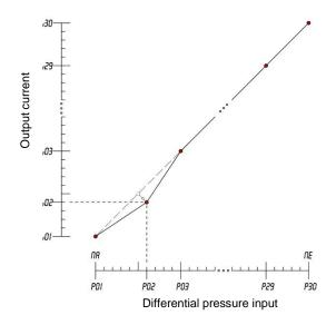
The table comprises 3...30 value pairs. For devices with a power output, the first value pair is  $\{.02|P02\}^1$ . The first value .02 defines the level of the output signal. The second value .02 determines the pressure at which the output signal is issued.
