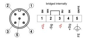
Connector 2 : Switching outputs
