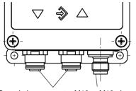
Round plug connector M12 M12 plug connection 5-pole flange socket
