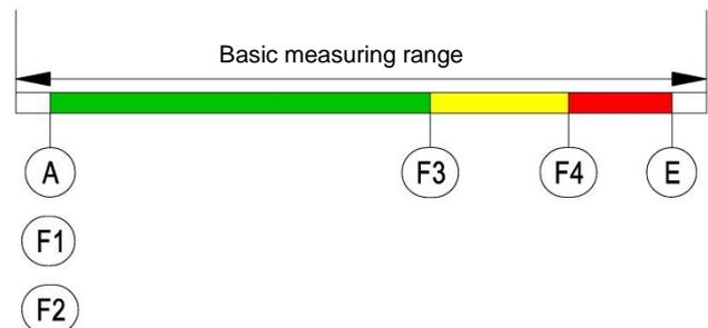
The parameter **Hysteresis** can be used to prevent fast and unwanted colour changes. The hysteresis is set in the range 0.1... 10%.
