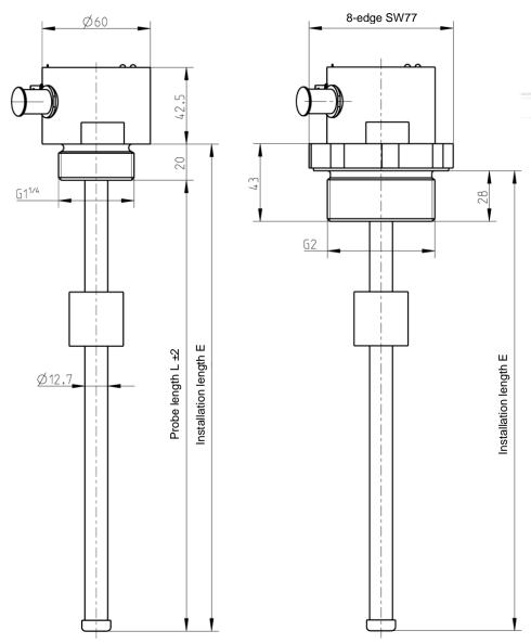
Installation length E = Probe length L + 20 mm
