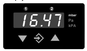
The 3.5 digit LCD display represents the current differential pressure in normal mode. The selected measuring unit is illuminated on the right of the display. (Note: The units shown on the screen may deviate from the actual version). Above the display the two light diodes • indicate the status of the switching outputs (LED shines = switch is closed).
