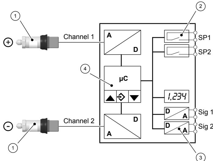
Fig. 3: Function diagram
