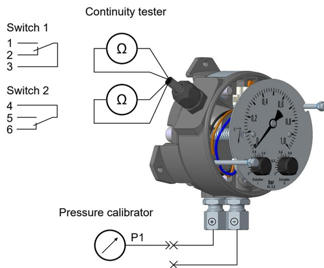
Fig. 4: Function test
