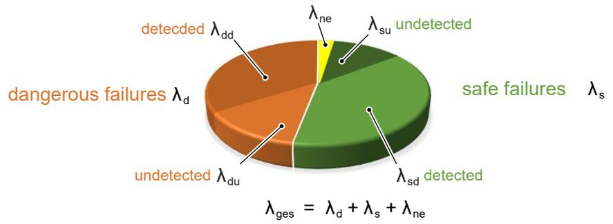
Fig. 8: Failure rates
