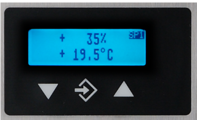
Fig. 10: Moisture/temperature display The FT61 is suitable for measuring moisture and the temperature of non-aggressive gaseous media.
